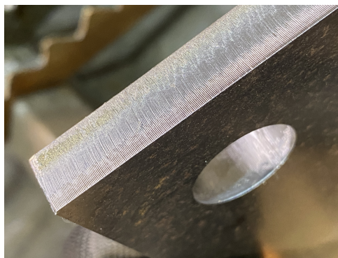
Figure 15. Sample Thickness = 10 mm; Roughness = 3.2 \mu\text{m} .
