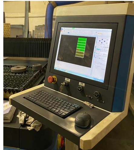
Figure 9. Machine control equipment.
